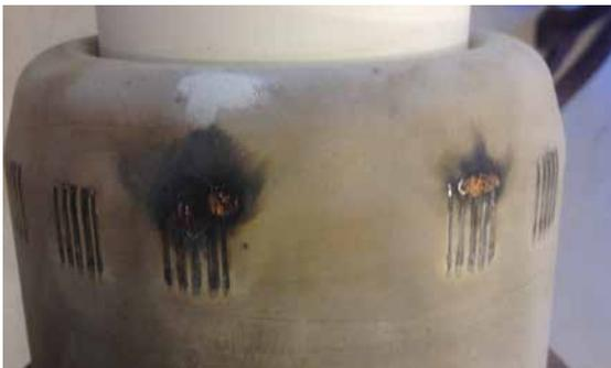
Flashover in the main contact carrier due to loose parts.
